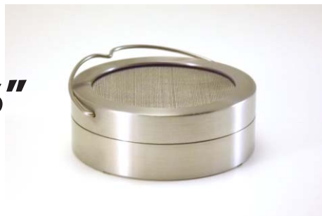
3" Large Capacity Holder (Material: SS316) - Cat# 8771C Interior 0.7" Ht x 3.0" I.D. (17.8 mm Ht x 76.2 mm I.D.) Exterior 1.05" Ht x 3.25" O.D. (26.7 mm Ht x 82.6 mm O.D.) Mesh Material: SS 316 / Mesh Size: 35x35 / Opening: 0.017" (0.43mm)
