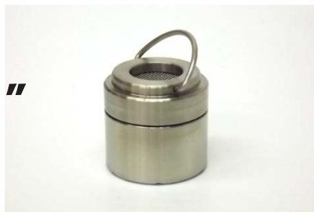
1" Large Capacity Holder (Material: SS316) - Cat# 8771A Interior 0.7" Ht x 1.0" I.D. (17.8 mm Ht x 25.4 mm I.D.) Exterior 1.05" Ht x 1.20" O.D. (26.7 mm Ht x 30.5 mm O.D.) Mesh Material: SS 316 / Mesh Size: 35x35 / Opening: 0.017" (0.43mm)
